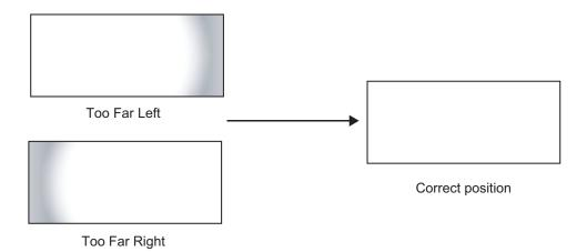
4. When the horizontal position is properly set, tighten the Yaw/X-Adjustment Levers to secure the lens in place.
